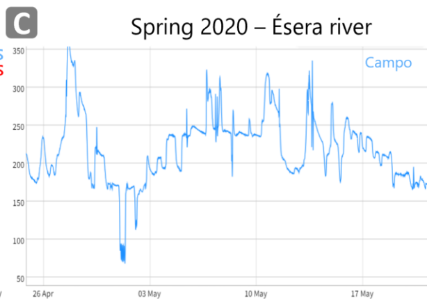
Figure 3.15: A Distribution of volumes classified as base, hydropeak, flood for each station annually and by season. B Extract of normalized spring flow data at Laspuña US (blue curve, bypassed reach) showing hydropeaks superimposed on a natural wave and Laspuña DS (red curve, downstream of HP) showing stable flows without peaks. C Extract of normalized flow data at Campo in spring 2020 showing a fully artificial hydrograph.
