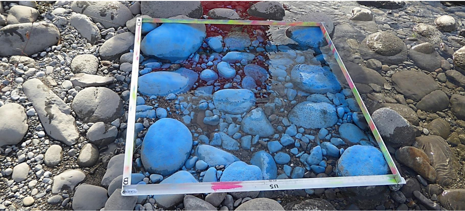
Bed grain size characterization of coarse bed at Laspuña reach (Upper Cinca River), 0.6 km downstream of hydropower plant. The size of the metal frame is 1m 2 , 01/11/2020. Author: Fanny Ville
