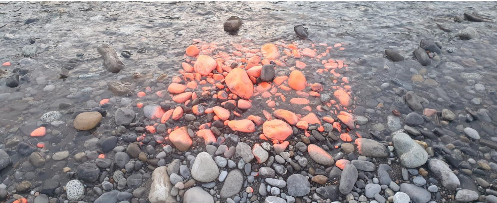
Bed grain mobility characterization at Ainsa reach (Upper Cinca River) 10 km downstream of hydropower plant, 01/11/2020. Author: Fanny Ville
