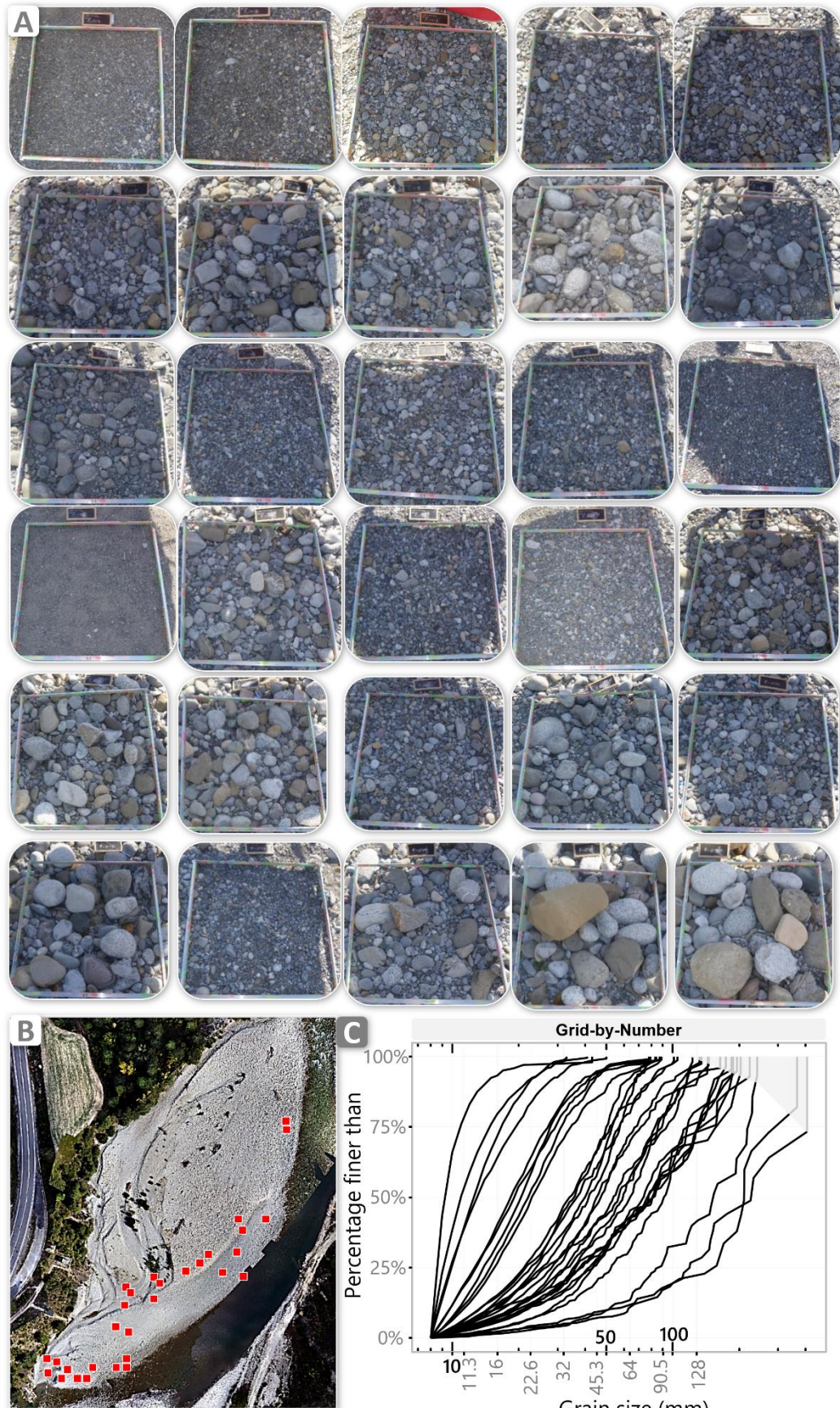
Figure 2.13: A Sampled patch. B Location of patches on the Escalona sediment bar. C GSD of the 30 patches sampled)
